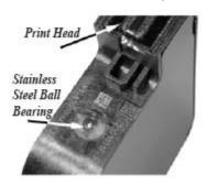
Important: If the cartridge rests on a paper towel to catch drippings, the printhead can touch the paper towel. Do not allow the printhead to remain on the towel for more than two minutes. This will prevent the
